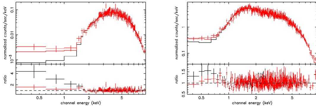
Figure 1. Left: XRT PC grade 0-12 spectrum of NGC 7172 using the new v009 (red) and previous v008 (black) response files. The use of a WABS\*POWERLAW model gives a value of  $N_H \sim 7.3 \times 10^{22} \text{ cm}^{-2}$ . Right: XRT WT grade 0-2 spectrum of the X-ray binary 4U 1608 using the new v009 (red) and previous v008 (black) response files. The use of a WABS\*(POWERLAW+DISKBB) model gives a value of  $N_H \sim 10^{22} \text{ cm}^{-2}$ .
