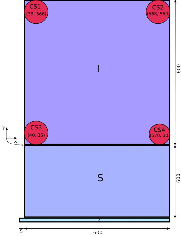
Figure A.1: Schematic of the *Swift*-XRT CCD22 identifying the imaging (I) and frame-store (S) sections, the readout register (R), and the  $^{55}\text{Fe}$  corner sources (CS). Charge is clocked in the parallel direction (Y), through both the imaging and frame-store sections, which have charge transfer inefficiencies  $CTI_{p,i}$  and  $CTI_{p,f}$ , respectively, and in the serial direction through the readout register with  $CTI_s$ .
