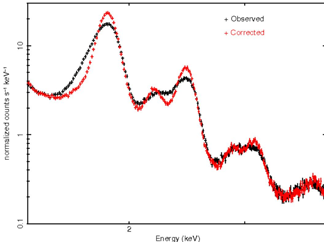
Figure C.6: Comparison of the observed and the trap corrected spectra extracted from a PC mode observation of the Tycho SNR from October 2009. The fit of the Silicon  $K\alpha$  line with an asymmetric Gaussian in IDL yielded a FWHM of  $179 \pm 8$  eV for the observed spectrum and of  $132 \pm 3$  eV for the corrected spectrum.
