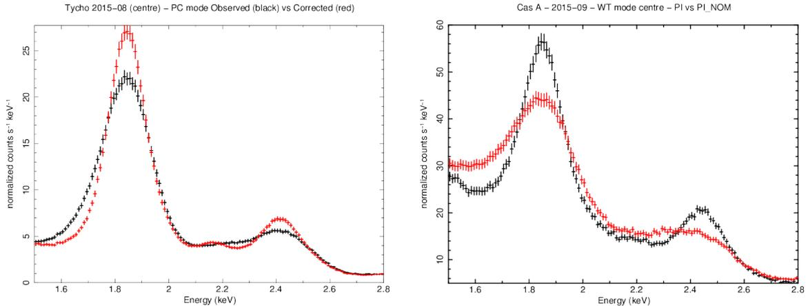
Figure 3: Comparison of non trap corrected spectra (in black) and trap corrected spectra (in red) in August 2015 Tycho observations taken in PC mode (left panel) and Cas A observations taken in WT mode (right panel).
