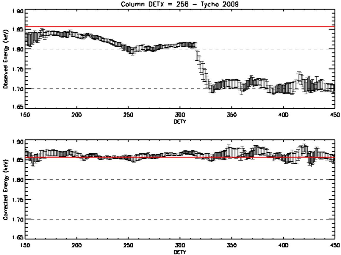
Figure C.5: In the top plot, a deep trap is identified in a Cas A Photon Counting mode observation in CCD column DETX=256 at DETY  $\sim$  310; in the bottom plot, the Si-K $\alpha$  line energy is restored after the trap correction has been applied.
