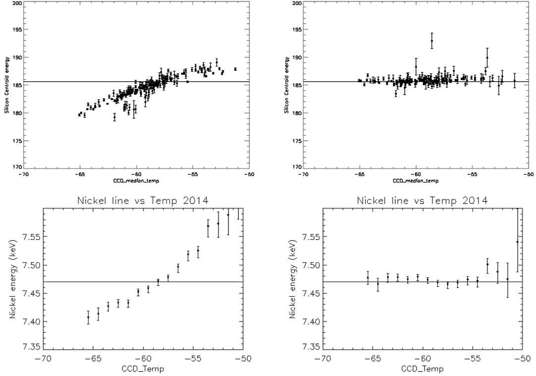
Figure C.9: The Tycho Silicon line (top left panel) and the instrumental Nickel  $K\alpha$  line (bottom left panel), in the data from the 2014-2015 campaign, show evidence of energy shifts from the expected values as a function of temperature. Processing the PC data with the updated gain file, that includes temperature dependent trap tables, the Gaussian fits in both cases give energies close to the expected values at all temperatures, as can be seen in the right panels.
