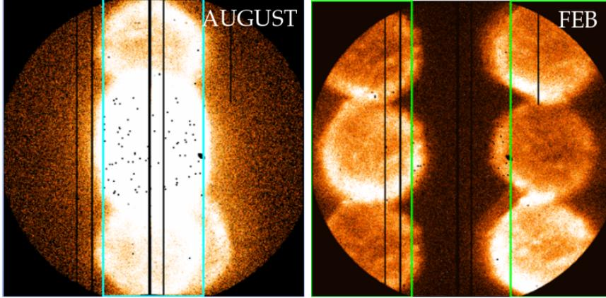
Figure 1: *PC trap mapping* - Observation strategy for the derivation of the new PC mode gain file `swxpcgains6_20010101v015.fits`, illustrated with the observations taken during the 2014-2015 campaign. During the summer/autumn epoch the Tycho SNR is positioned to cover the central strip of the CCD (*left panel*), while during the winter/spring epoch the observations cover the left and right sides of the CCD (*right panel*).
