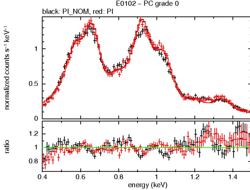
Figure C.8: Observed (black) and trap-corrected (red) spectrum of E0102 used to determine the CTE energy dependence at low energies. Dataset from 2008 to 2010 were merged to extract the spectra, and grade 0 events were selected. There is a definite improvement of the lines around 0.675, 0.915 and 1.035 keV in the trap corrected spectrum.
