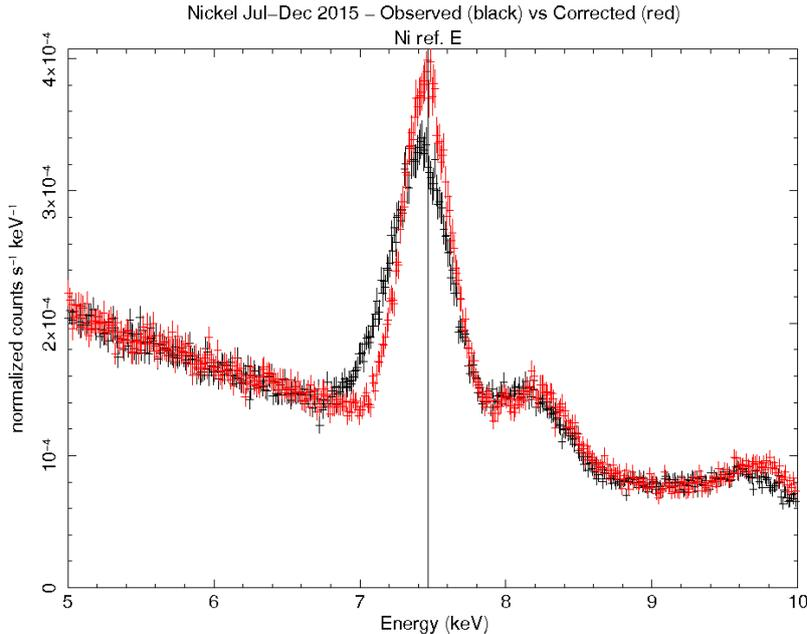
Figure 4: Nickel line extracted from PC observations collected between August 2014 and December 2015 with exposure greater than 100 seconds. The trap corrected spectrum (in red) shows a recovery of the line flux and an improvement of the energy resolution in comparison to the observed spectrum (in black). The vertical line shows the reference energy for the Nickel line (7470 eV).
