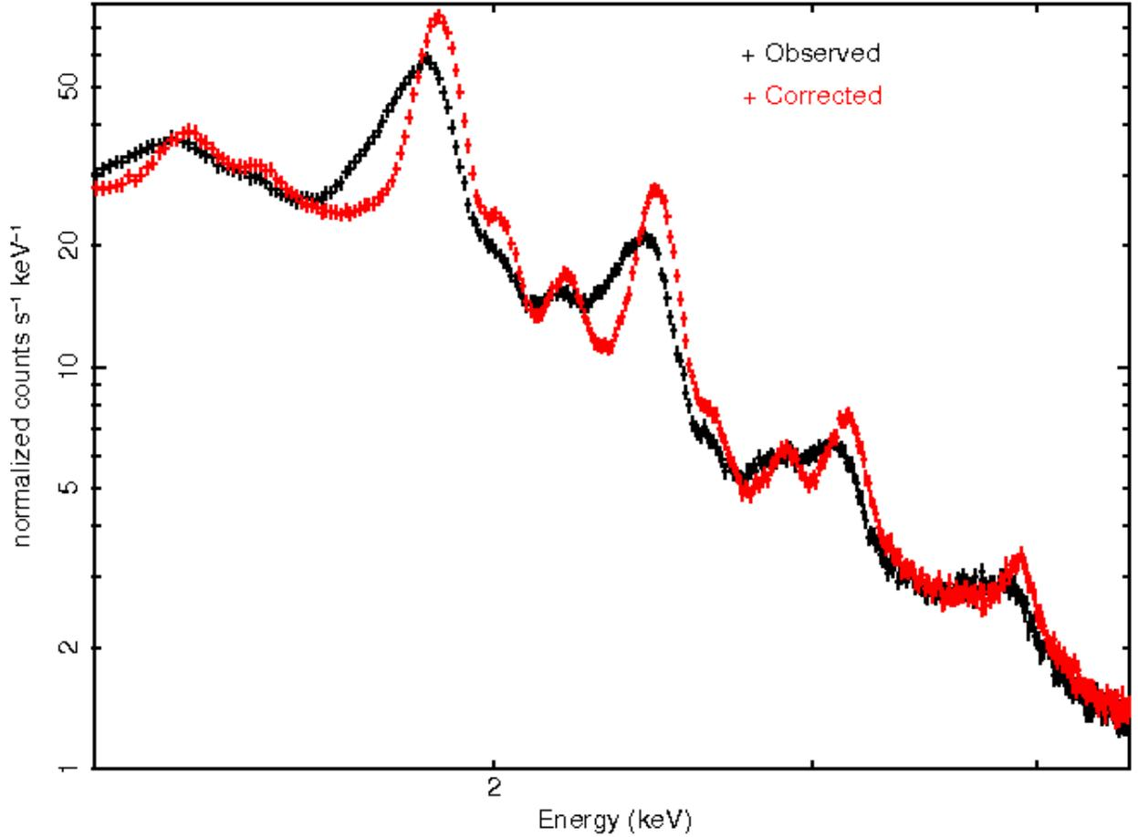
Figure C.7: Comparison of the observed and the trap corrected spectra extracted from WT observations of the Cas A SNR in October of 2007. The fit of the Silicon  $K\alpha$  line with an asymmetric Gaussian in IDL yielded a FWHM of  $152 \pm 13$  eV for the observed spectrum and of  $106 \pm 3$  eV for the corrected spectrum.
