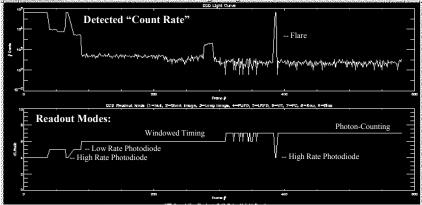
Top Panel: onboard estimate of count rate vs time, log scale, from data run at Panter calibration facility. using simulated GRB lightcurve.
