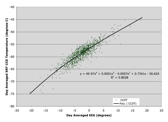
Figure 1. An updated model for estimating the XRT CCD temperature as a function of Earth Elevation Angle.
