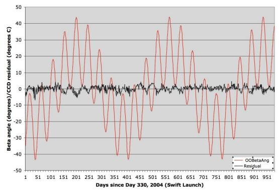
Figure 2. Residuals from the model show in Figure 1 (black) and the  $\beta$ -angle (sinusoidal line) for the first 1000 days of XRT operation.
